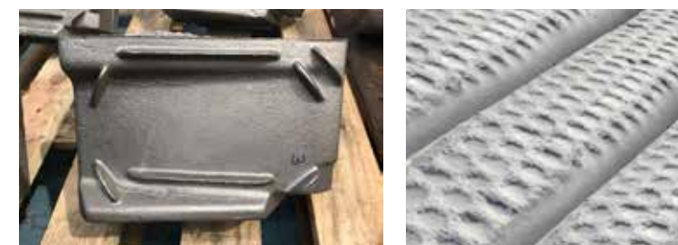
VSI Crusher, with ceramic inserts
