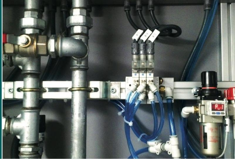
The ESTANDA automatic Water Injection System ensures the consistency of the mill internal working temperature. In order to provide the appropriate equipment supply for your mill, it will be necessary first of all to carry out a thermal heat balance study of the mill.
